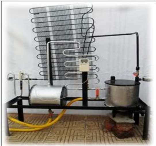
Fig.2 Complete view of vapour absorption refrigeration system.
