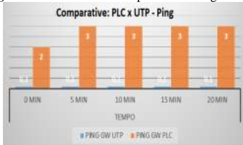
Figure 18. Test result PING parameter for gateway
