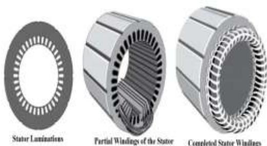
**Figure 2.3** Stator Windings construction through laminations
