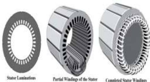
**Figure 2.3** Stator Windings construction through laminations
