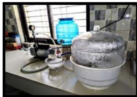
Fig-3: RCPT of concrete samples.
