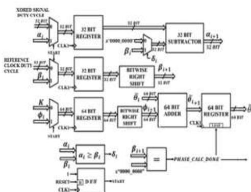
Fig.5. Architecture of phase value computation
