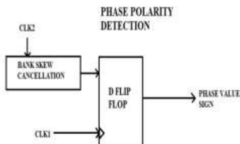
Fig.6. Architecture of phase polarity detection
