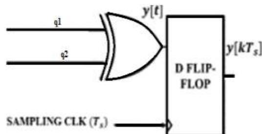
Fig.3. Architecture of XOR based phase detector
