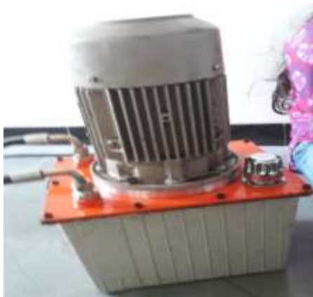
Fig 1. Oil Tank of the power pack unit
