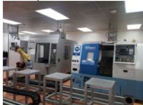
Fig.7. Integral system of CNC equipment for the reproduction and manufacture of test tube in different materials.
