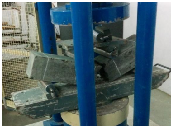
Fig.6 Failure of Beam
