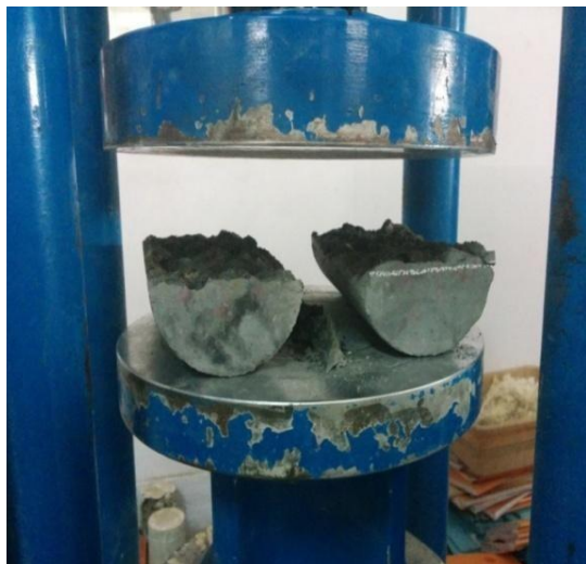
Fig.4 Failure of Cylinder
