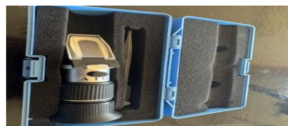
Figure 2. Refractometer used to carry out the tests for the determination of °Brix degrees
