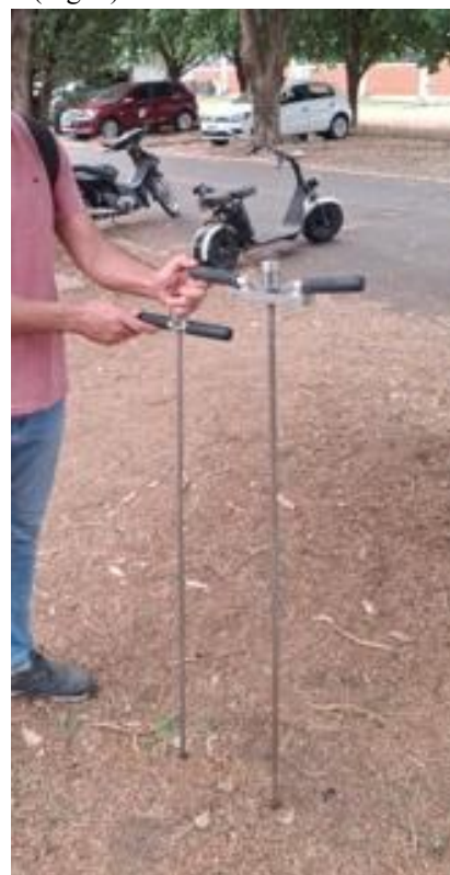
Fig. 5. General view of the probe used for sampling the radon and thoron from the surficial soil layers located at the Geology Department, IGCE-UNESP-Rio Claro Campus.
