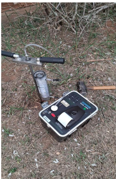
Fig. 6. Probe coupling to RAD7 equipment during sampling the radon and thoron from the surficial soil layers located at the Geology Department, IGCE-UNESP-Rio Claro Campus.
