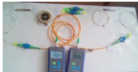
Fig. 3. Set-up based with Hybrid Mach-Zehnder interferometer
