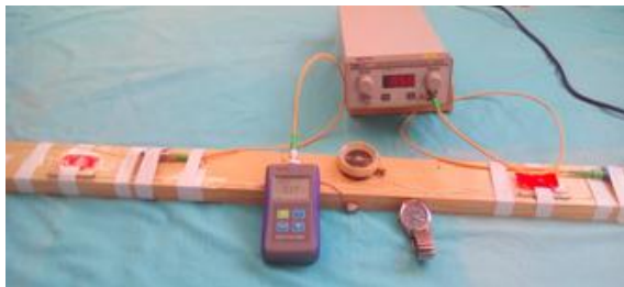
Fig. 5. Experimental set-up based on Mach-Zehnder interferometer
