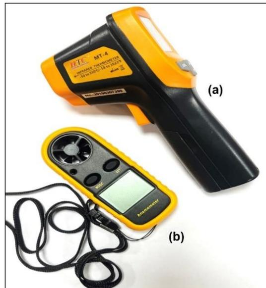
**Fig. 6.** Image of the used (a) IR digital thermometer (b) anemometer.
