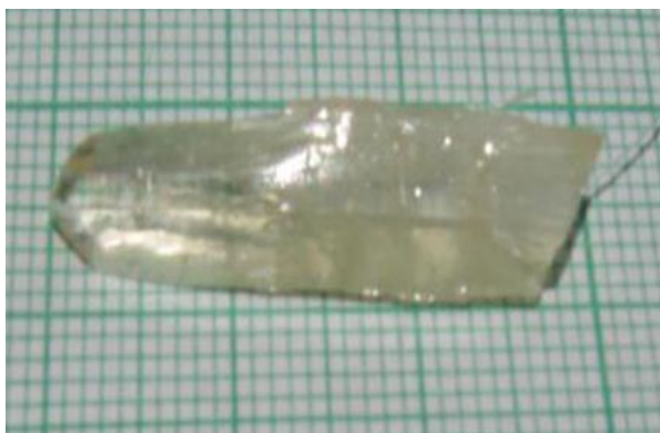
Fig 1(b): grown crystals of CTSTM by slow cooling method.
