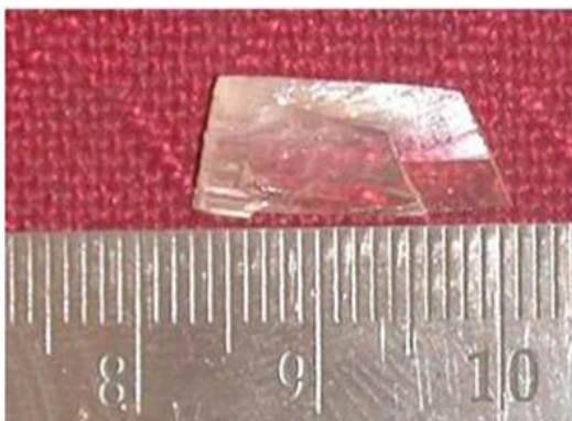
Fig 1(a) grown crystals of CTSTM by slow cooling method.
