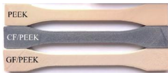
Fig.5 Variants of PEEK material dog bone structure [4]
