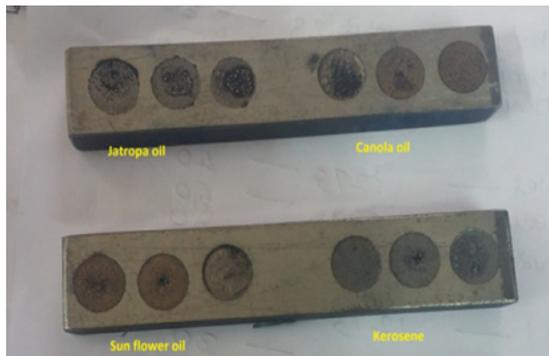
Fig 6 Machined samples with copper electrode.[10]
