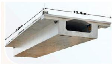
Fig 1: Full Span Box Girder
