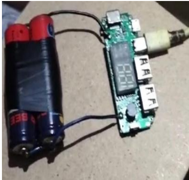
Fig6.ConnectionOfCircuitWithLI-IONBatteries and Power Bank Module
