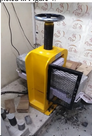
Figure 4 : Flexural strength test.
