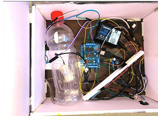
Figure 30: - Inside view of Floor cleaning robot (connections)
