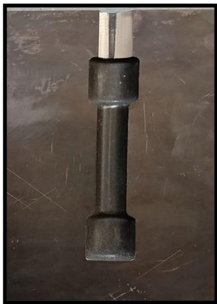
Fig. 8: Shows the Die of Tensile Specimen.
