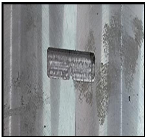
Fig: 5 Impact Specimen Mould According to ASTM E-23 Standards.
