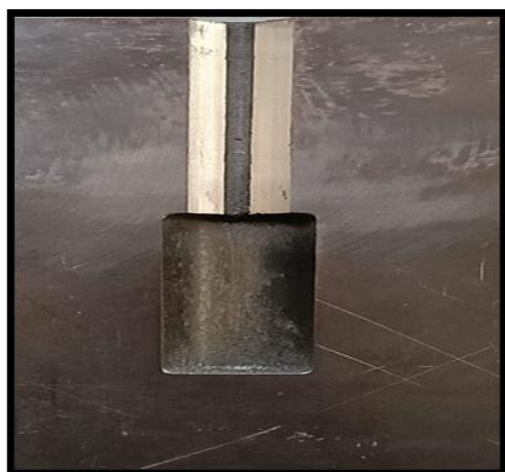
Fig. 10: Shows the Die of Compression Specimen.
