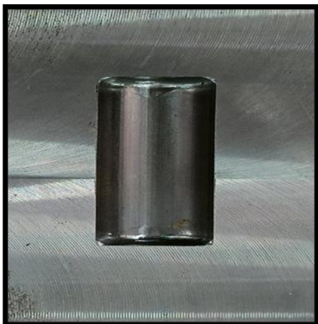
Fig: 4 Compression Specimen Mould According to ASTM E-9 Standards.
