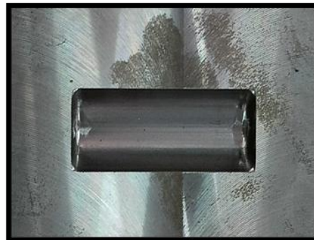
Fig: 6 Hardness Specimen Mould According to ASTM E-10 Standards.
