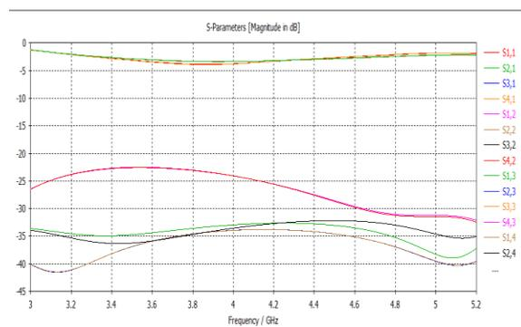
Fig. 9 Scattering parameters of Dual band 4X4 MIMO antenna
