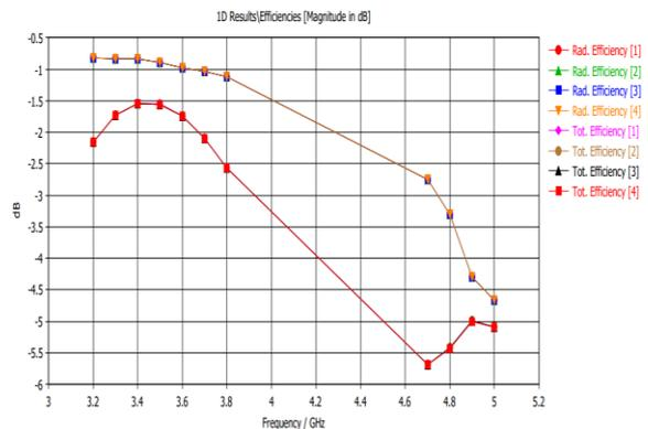
Fig. 10 Power variations of Dual band 4X4 MIMO antenna
