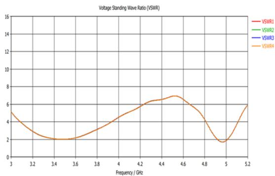
Fig. 5 Voltage Standing Wave Ratio of Dual band 4X4 MIMO antenna
