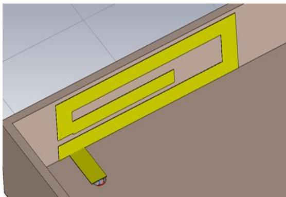
Fig. 2 4X4 Dual Band Antenna design using CST Studio Software
