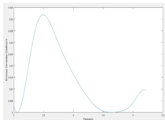
Fig. 11 Envelope Correlation Coefficient of Dual band 4X4 MIMO antenna
