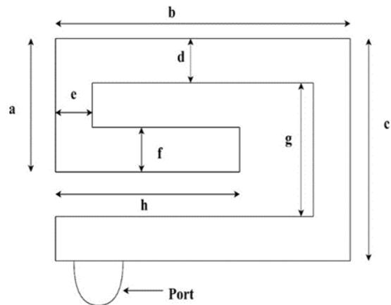
Fig. 1(a) Antenna element model Main view
