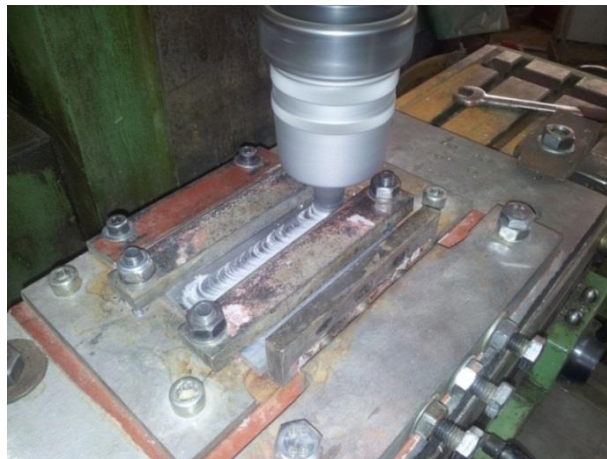
Figure 4: Clamping of the plates and the friction stir welding process
