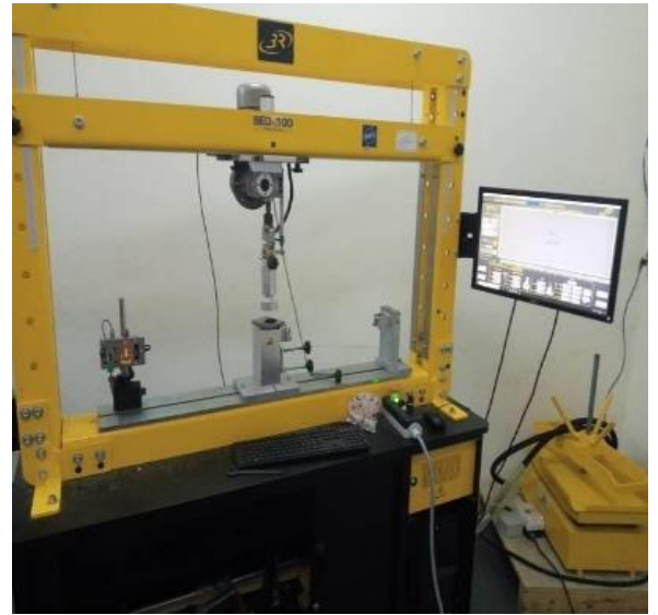
Figure 1: compression test set-up
