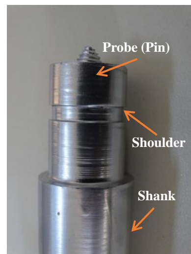
Fig. 2 Photograph of FSW tool showing its different parts
