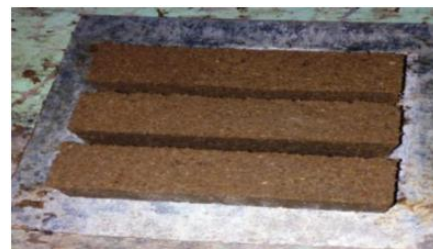
Figure 2: mortar samples composed of sand and geopolymer binder
