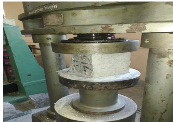
Fig. 1. Compressive tests on Geopolymer concrete
