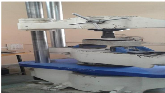
Fig. 4. The testing setup for the beam sections
