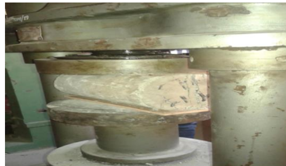
Fig. 6. Split tensile Test on Geopolymer Concrete
