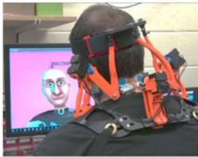
Fig.1.2 Three-degree-of-freedom dynamic neck collar
