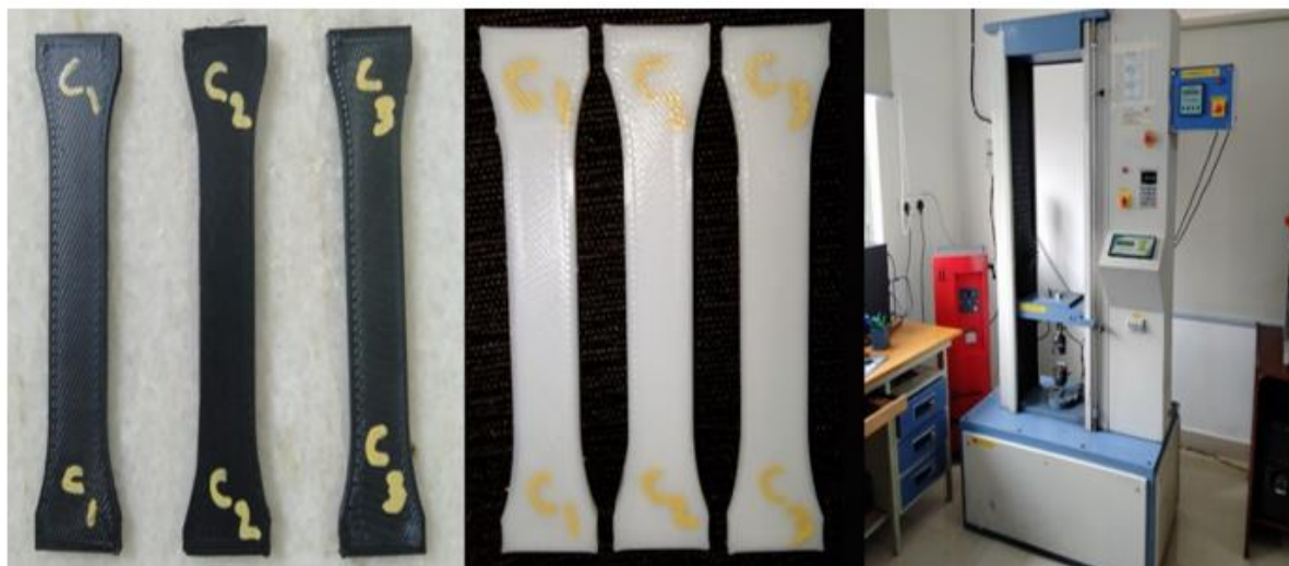
Figure 2.4 Images of all components of compressive test; PLA specimens b) ABS specimens c) experimental setup
