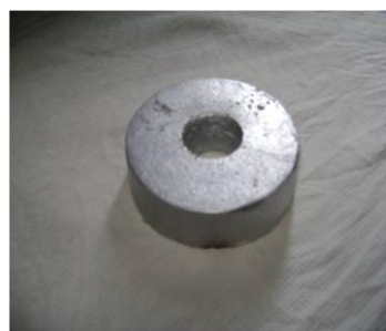
Fig 2. A Casted Aluminum alloy 356 gear blank
