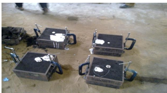
Fig 1. Green sand casting of Aluminum alloy 356 gear blanks
