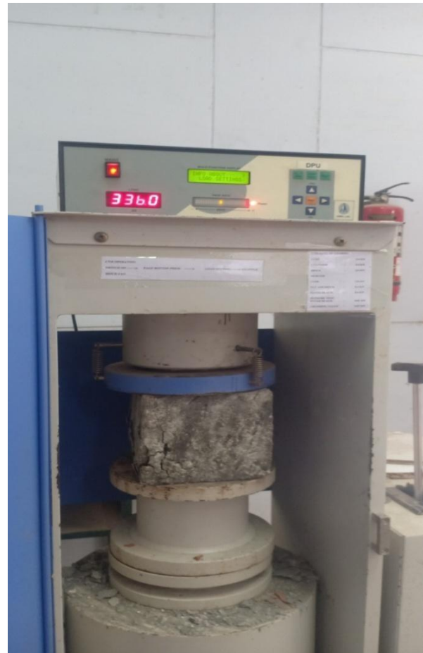
Testing of concrete by compressive testing machine
