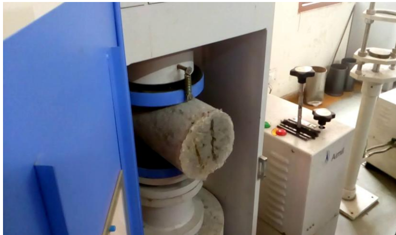
Split tensile strength test
