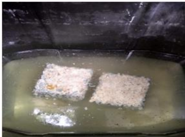
Cubes immersed in acid solution
