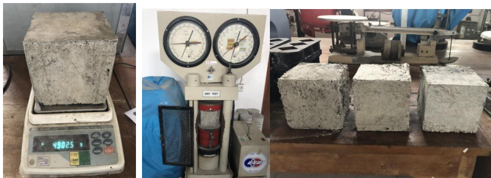
a. Weight Test b. Compression Test c. Cube Condition After Compression Test Figure 4, Manufacturing Results of Local Sawdust Panels
