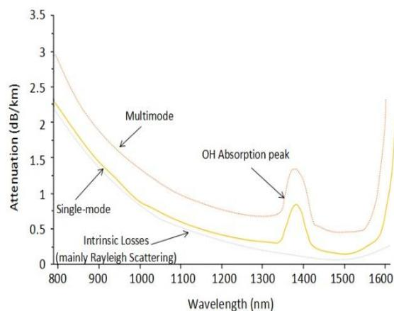
**Figure 3:**Optical fiber absorption.
