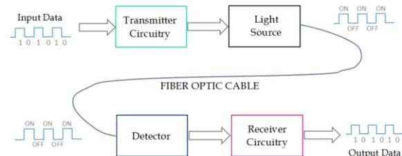
Figure 1: Main components of the optical fiber network.
