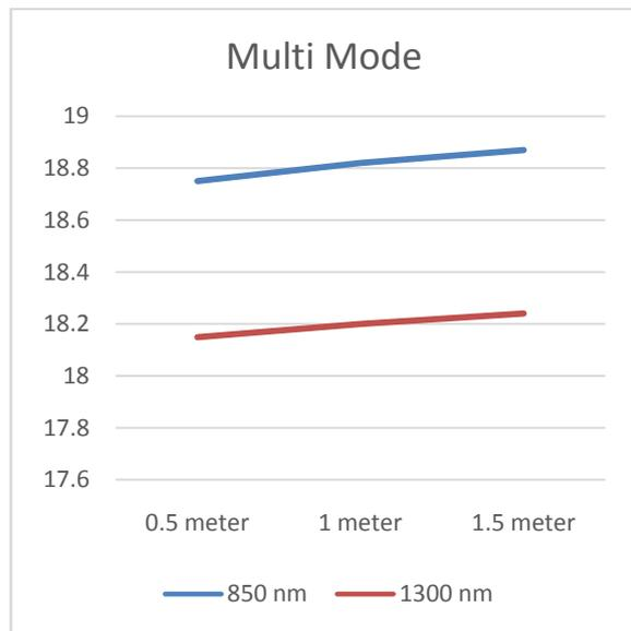
**Graph2:**The relationship between wavelength and luminous intensityMulti mode optical fiber.
