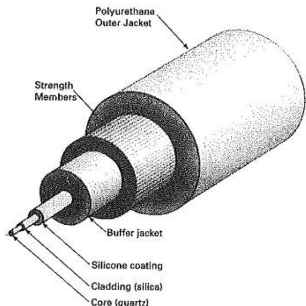
Figure 2: The six main components.
