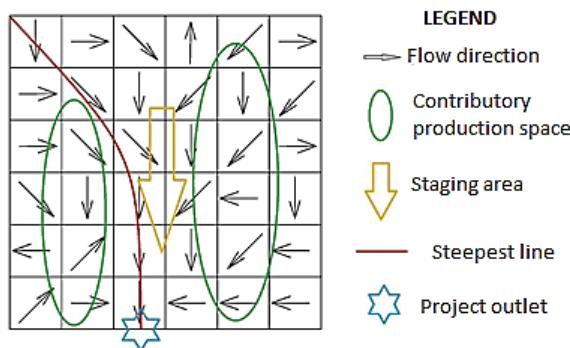
Figure 2: Flow Direction Models
