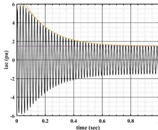
Figure 5. Three phase fault current for ‘min fault current’
