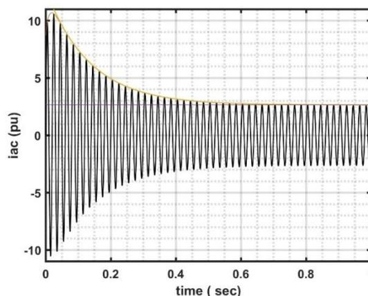
Figure 6. Three phase fault current for ‘rotor min vibration’
