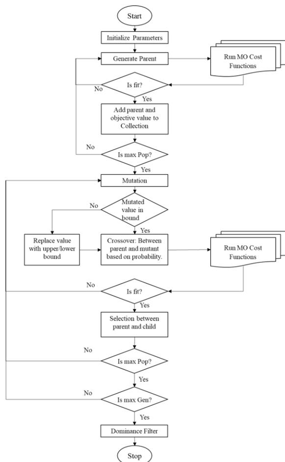
Figure 1. Flow Chart for the Computer Program (MODE).
