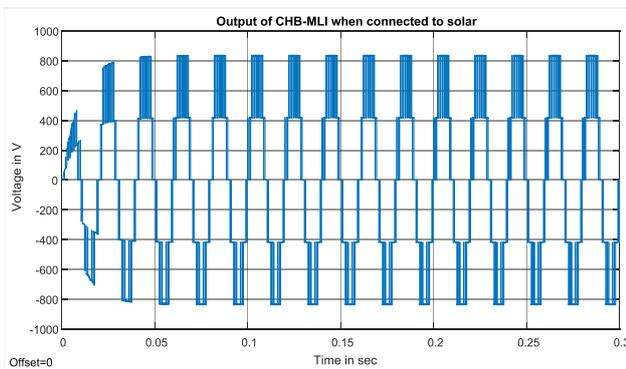
Fig. 11. Output voltage of single phase 5-level CHB-MLI for using PV system
