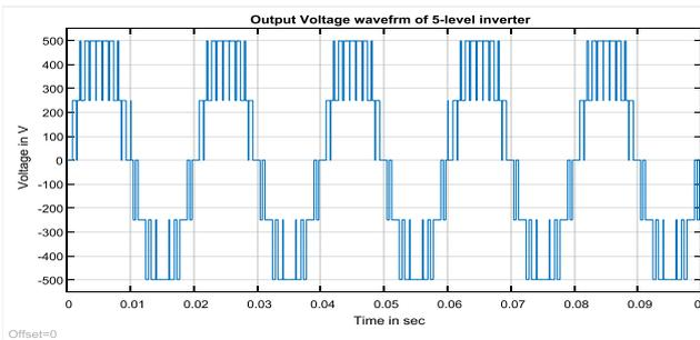
Fig. 6. Output voltage of single phase 5 level CHB-MLI
