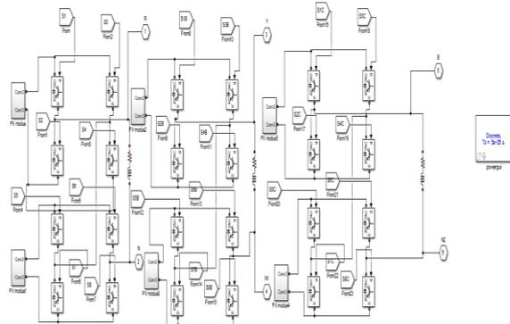
Fig. 16. Simulation model of PV connected across CHB-unit
