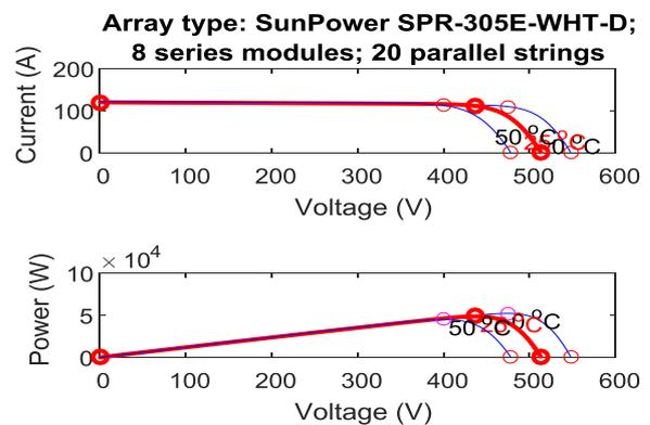
Fig. 8. PV-VI characteristics of PV system
