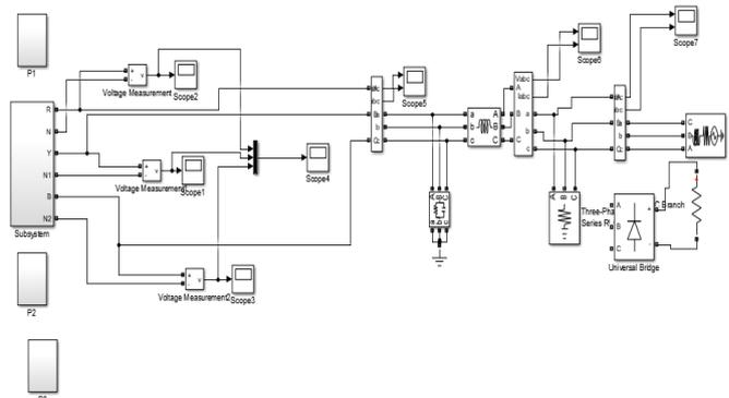
Fig. 15. Simulation model of CHB-MLI based PV system
