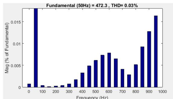
Fig. 20 THD analysis of Output voltage of Solar system grid.
