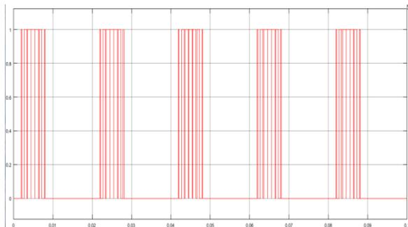
Fig.10. Switching responses of In Phase Disposition PWM (IPDPWM)
