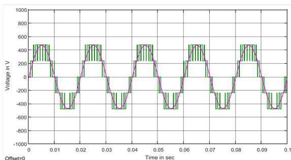
Fig. 17. Inverter phase-to-phase output voltage and its fundamental component
