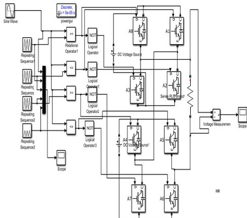
Fig. 5. Simulation model of proposed CHB-MLI
