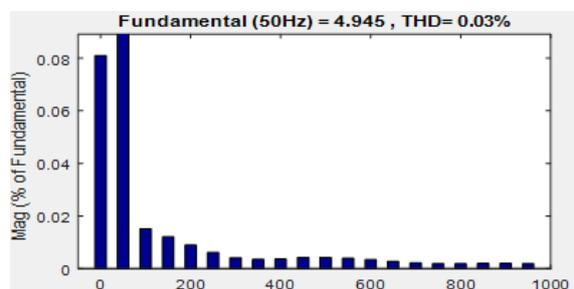
Fig. 21 THD analysis of Output Current at grid side
