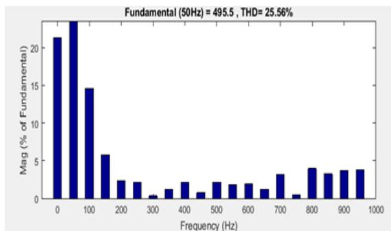
Fig. 12. THD of voltage output of CHB MLI
