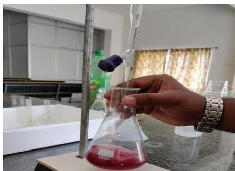
Fig.1 hardness test
