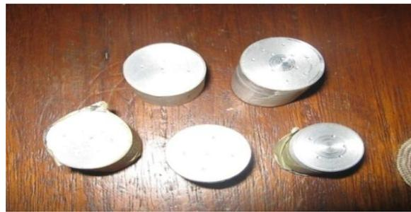
Figure 3: Specimen Samples for Hardness Tests
