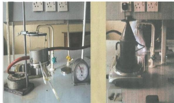
Figure 8: Experimental Set-up for Thermal Conductivity Test
