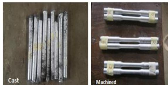
Figure 5: Samples of Tensile Test Specimen.
