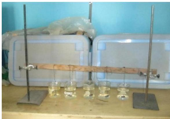
Figure 9: Experimental Set-up for Corrosion Measurement
