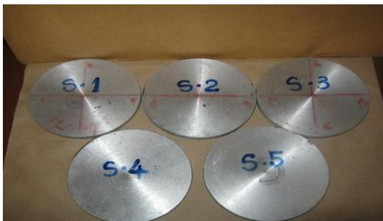
Figure 7: Samples of Machined Thermal Conductivity Test Specimen
