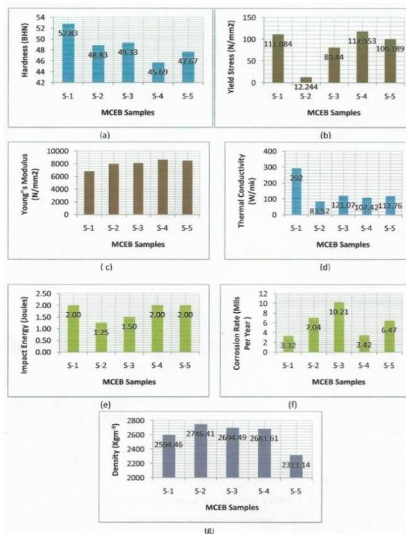
Figure 10: Test results for (a) Hardness (b) Yield Strength (c) Modulus of Elasticity (d) Thermal Conductivity (e) Impact Strength (f) Corrosion Rate and (g) Density
