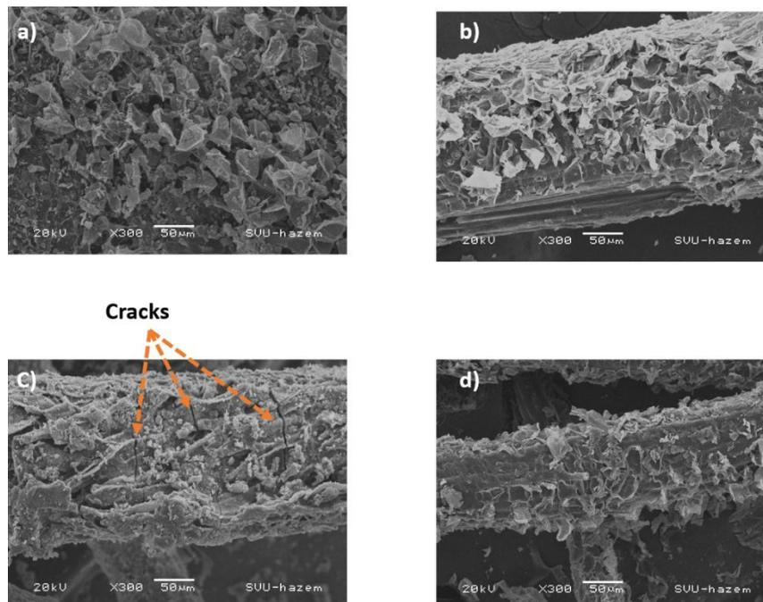
Figure 7 SEM photograph at 2 hr of a) Date palm tree (DPT) without treatment b) With HCl c) with NaOH3 d) with  $\text{CH}_3\text{COOH}$  at 10 %
