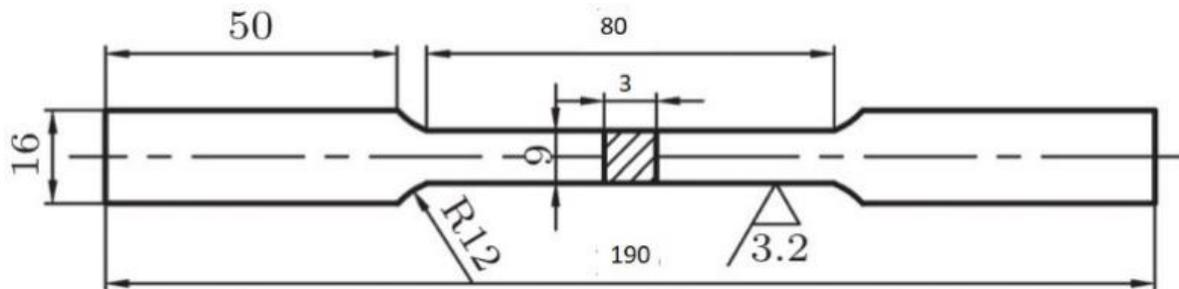
Figure 4 schematic drawing of the tensile test specimen
