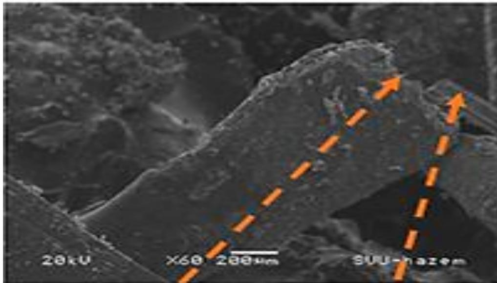
**fiber breaking and rubber pull out**
