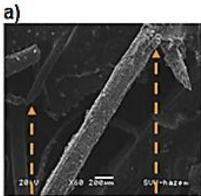
**Rubber tearing and Fiber bridging and pull out**
