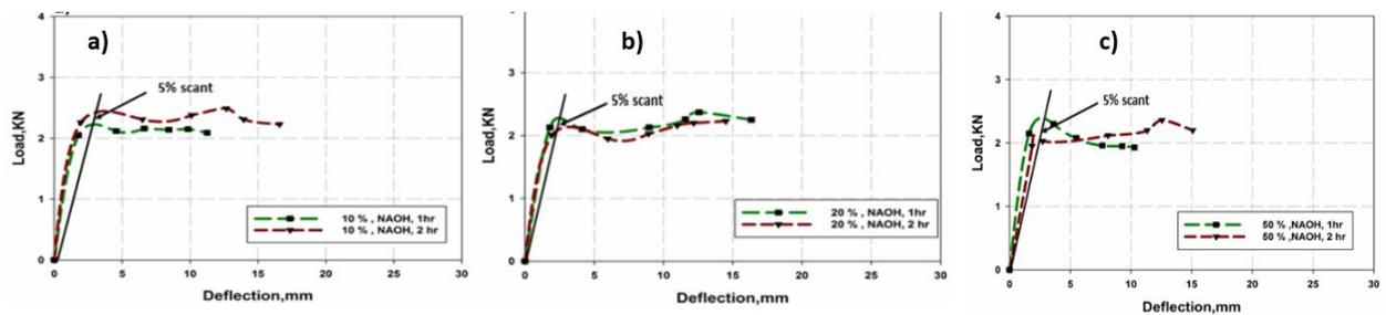
Figure17. Load- displacement relation in compact tension test of DPTRE with rubber at NaOH treatment in temperature 100C°for 1hr,2hr at concentration a) 10 %, b) 20 %, c)50%.
