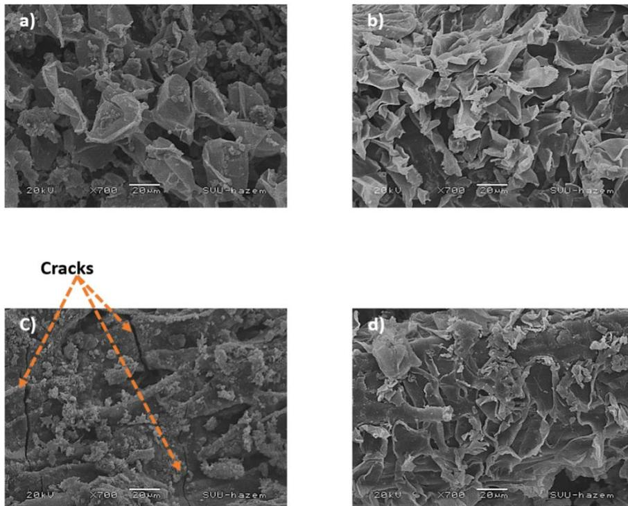
Figure 6 SEM photograph at 1 hr of a) Date palm tree (DPT) without treatment b) With HCl c) with NaOH3 d) with CH<sub>3</sub>COOH at 10 %
