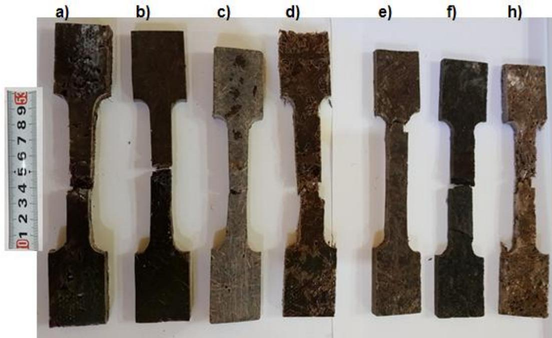
Figure 15 Failure Modes of some samples of DPT with rubber of tensile specimens (a,b) HCl,(c,d,e) NaOH, (f,h) CH<sub>3</sub>COOH
