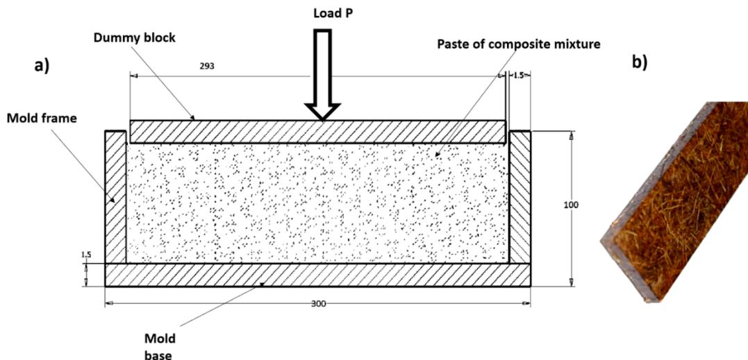
Figure 3 manufacturing set up; a) Compaction molding, b) Date palm tree product
