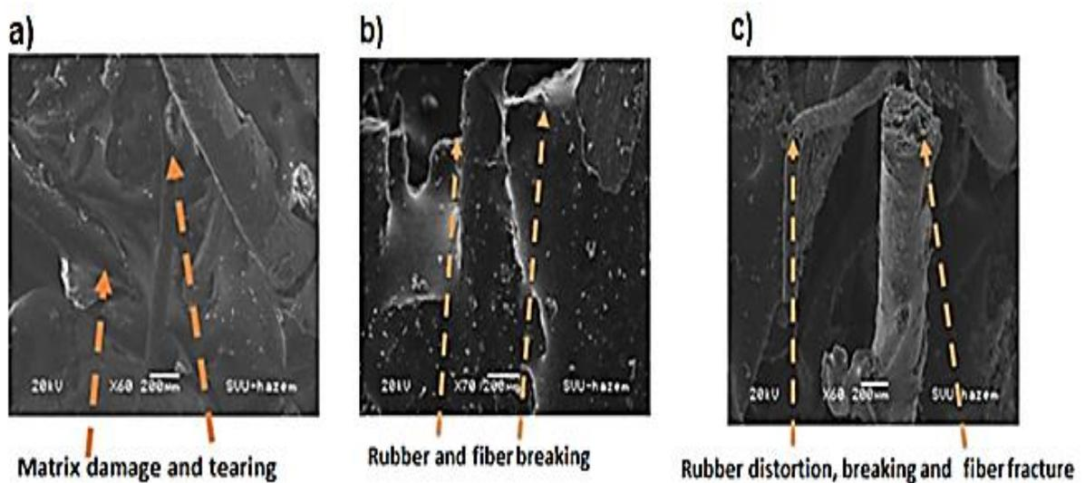
Figure 12 SEM photograph date palm tree with rubber and treatment at 100°C with a) NaOH, 10% .b) with NaOH, 20%, at 1hr. c) with NaOH, 50%, at 1hr.
