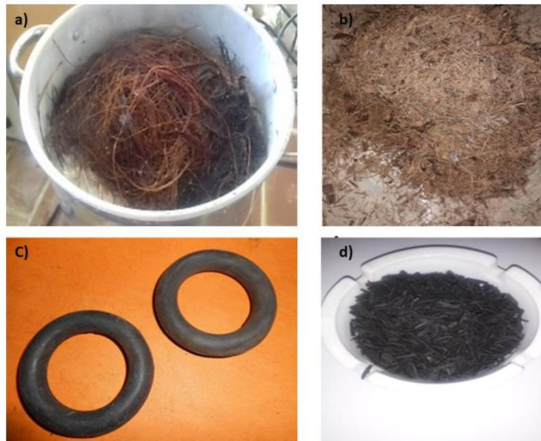
Figure 2 Renifircement phase a) Fiber bundles; b) Chopped Fibers; c) Rubber from car tires; d) Cut rubber
