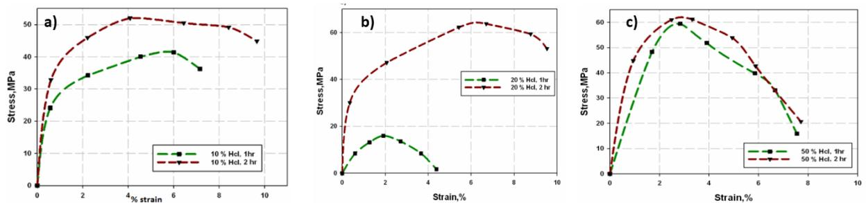
Figure 8 Average Stress strain relation of DPTRE with rubber at HCl treatment in temperature 100°C for 1hr, 2hr at concentration a) 10%, b) 20%, c) 50%
