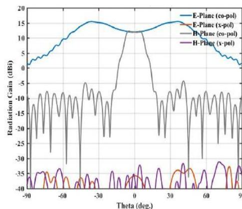
Figure 3(a): Simulated radiation pattern of optimized Lens
