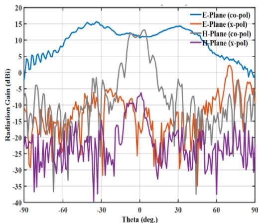
Figure 3(b): Benchmark measurement radiation pattern of optimized Lens
