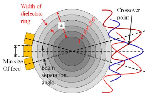
Figure 1: Conceptual design architecture of Luneburg lens for beam optimisation
