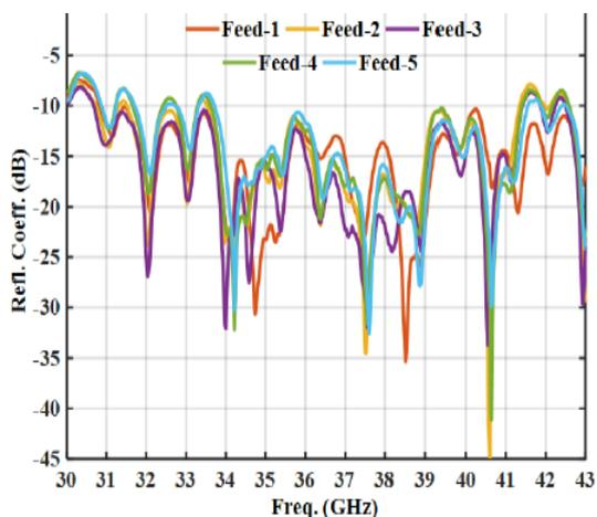
Figure 4(b): coefficients of reflection measured
