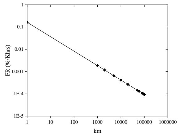
Figure 2. Failure rate at different Km.
