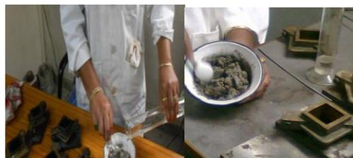
Figure.1. Preparation of Geopolymer Mortar Mix.
