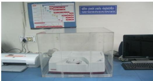
Figure.5. Fourier Transform Infrared Spectrometer FT-IR.
