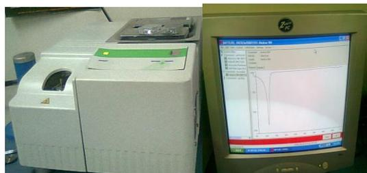
Figure.7. Differential Scanning Calorimeter (DSC).
