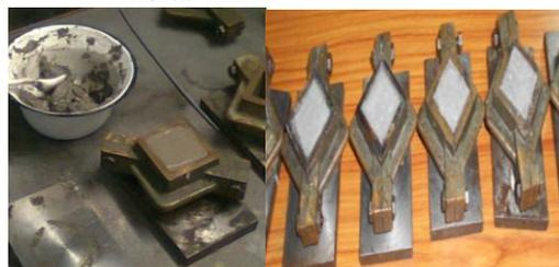
Figure.2. Casting of Geopolymer Mortar Cubes.
