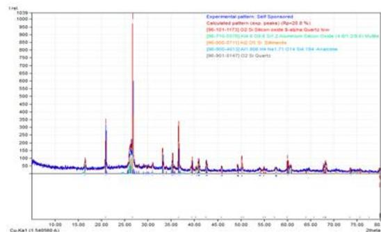
Figure.10. XRD Pattern of Geopolymer Mortar Cube.
