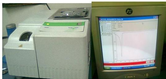
Figure.7. Differential Scanning Calorimeter (DSC).
