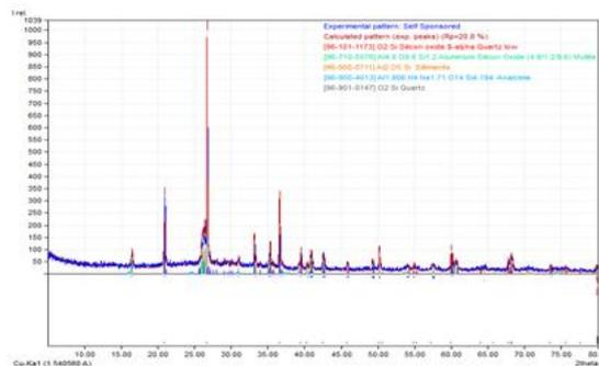
Figure.10. XRD Pattern of Geopolymer Mortar Cube.
