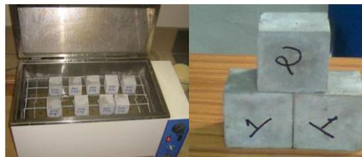
Figure.3. Curing of Geopolymer Mortar Cubes.
