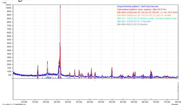
Figure.9. XRD Pattern of Fly Ash.
