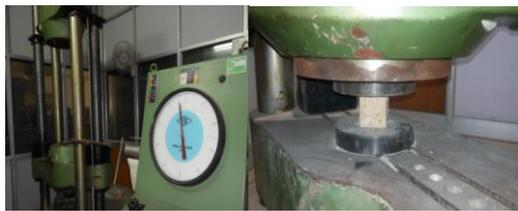
Figure.4. Compressive Strength Test with UTM.
