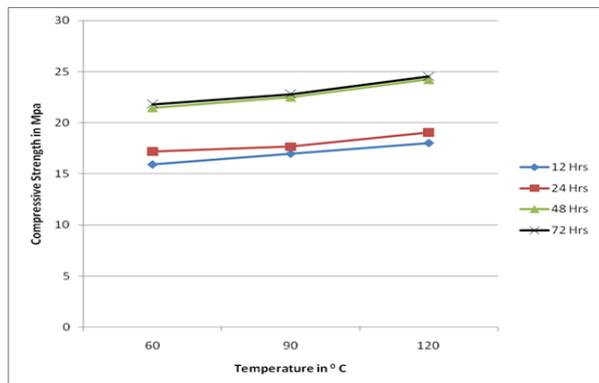
Figure.8. Compressive strength with different curing time and Temperatures.
