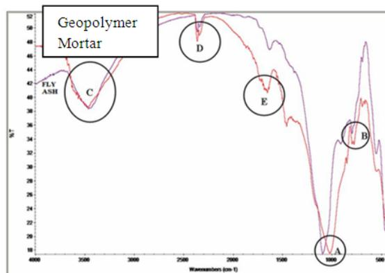
Figure.11. FT-IR Pattern of Fly ash and Geopolymer Mortar Cube.
