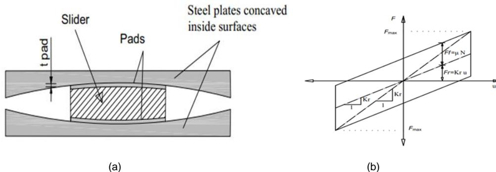
Fig. 1.(a) Double curved slider; (b) force-displacement (hysteresis) diagram [14]
