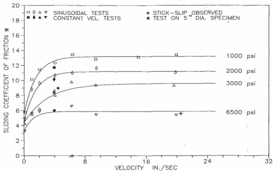
Fig. 2. Sliding friction coefficient variation with velocity of Glass-Filled Teflon at 25% for sliding parallel to Lay [23].
