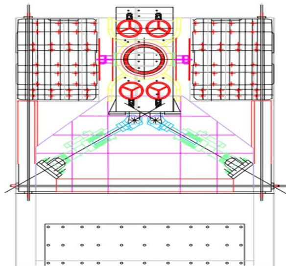
Fig. 3. The bearing tester (plan scheme).
