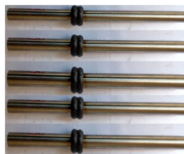
Fig 3: NiTiNol rods welded
