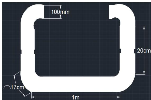
Fig.2 Dimensions of PVC recirculation pipe.
