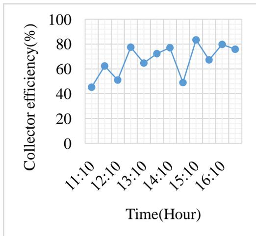
Fig. 9 Collector efficiency versus drying time.
