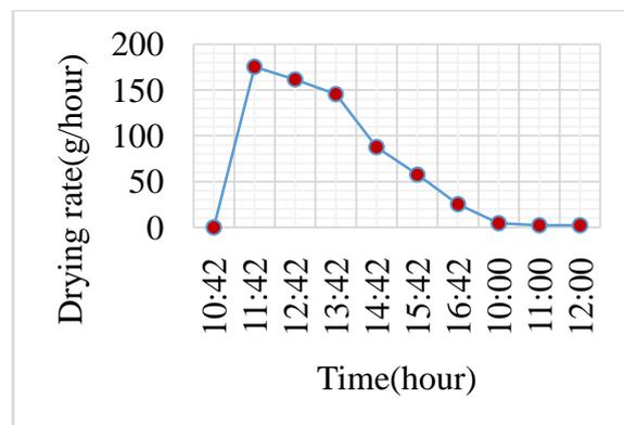
Fig.16 Drying rate versus time graph of tomato.
