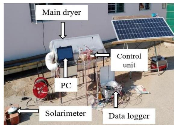
Fig. 7 No-load experimental setup without heater.
