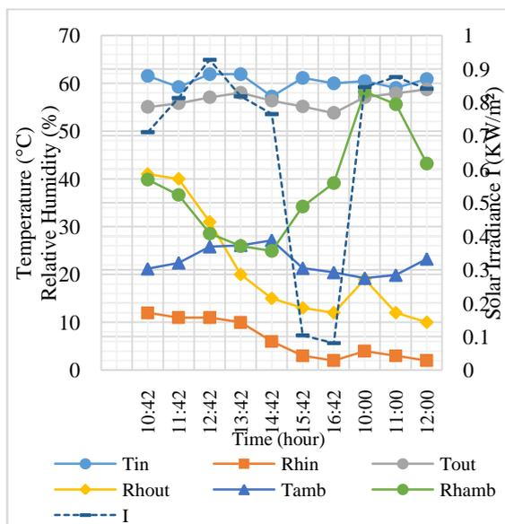
Fig. 12 Temperature, relative humidity, and solar irradiance against the time of drying.
