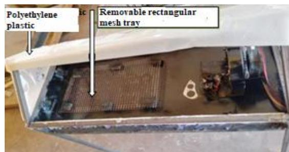
Fig.3b Internal view of the solar tunnel dryer.
