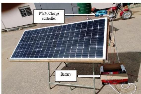
Fig. 5 Ground-mounted PV system.
