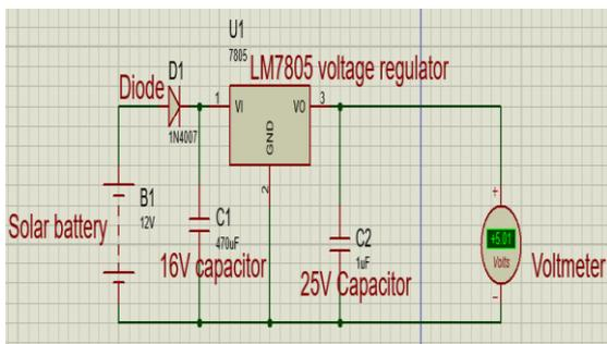
Fig. 4b 12V/5VDC Voltage Stabilizer.
