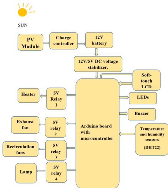
Fig. 6 Block diagram of the general principle of operation.
