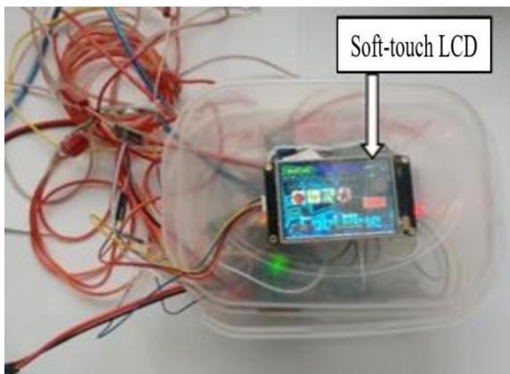
Fig. 4a Fabricated automatic optimum temperature monitoring and control unit.
