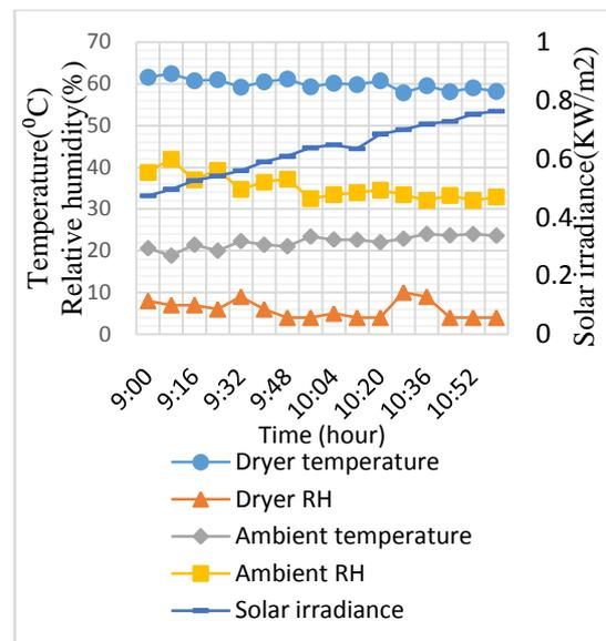
Fig.10. No-load experiment with heater and control.
