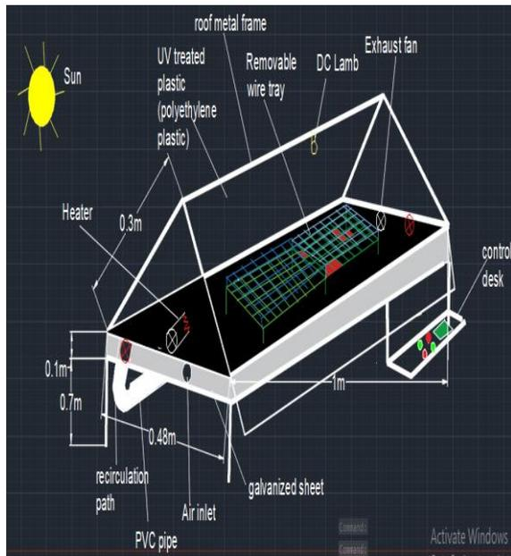
Fig. 1 AutoCad design of the dryer.
