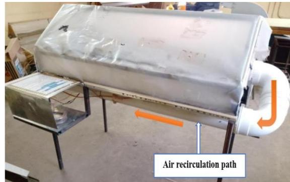
Fig.3a Outside view of solar tunnel dryer with air recirculation pipe.
