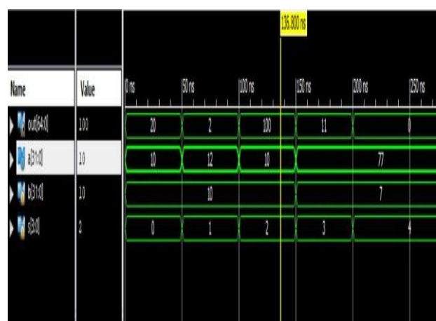
Fig 2: Simulation Outputs for 32-bit floating point ALU
