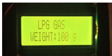
Figure 5: System displaying the weight of the cylinder on Lcd display
