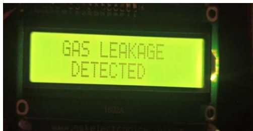
Figure 6: System displaying the leakage of cylinder on LCD display
