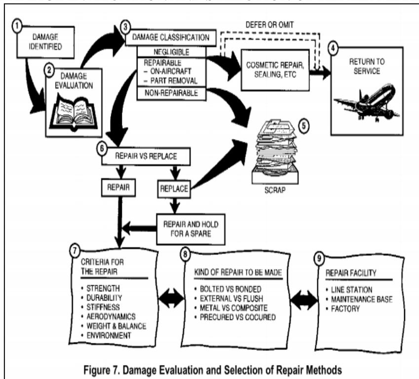
Figure 7. Damage Evaluation and Selection of Repair Methods
