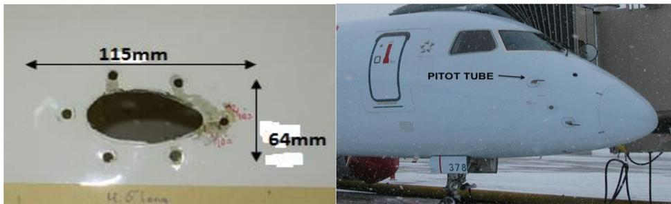
Figure 1: Damage Description and Repair Location on Fuselage Skin
