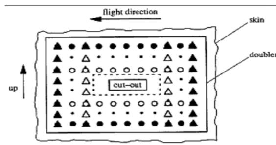
Figure 2: Repair Sketch for the Crack Damage
