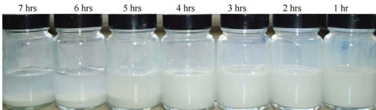
Fig.3 Sedimentation of Al 2 O 3 nanoparticles without stabilizer [86]
