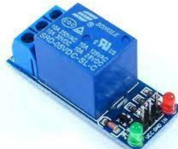
Figure 5: The Relay Module
