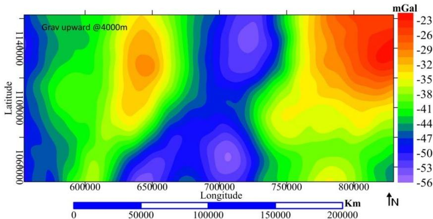
**Figure 7:** Upward Continued Bouguer Gravity Map at 4000m (mgal)
