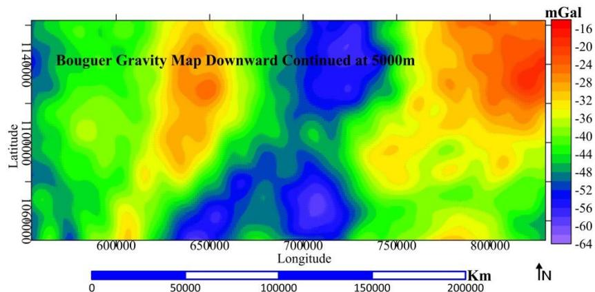
**Figure 10:** Bouguer Gravity Contour Map Downward Continued at 5000m (mgal)
