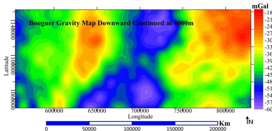
Figure 9: Bouguer Gravity Map Downward Continued at 4000m (mgal)
