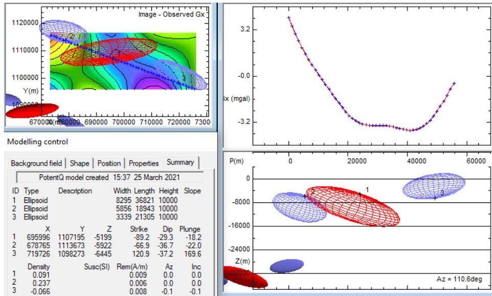
Figure 15: Profile 4 with R.m.s difference = 0.020%
