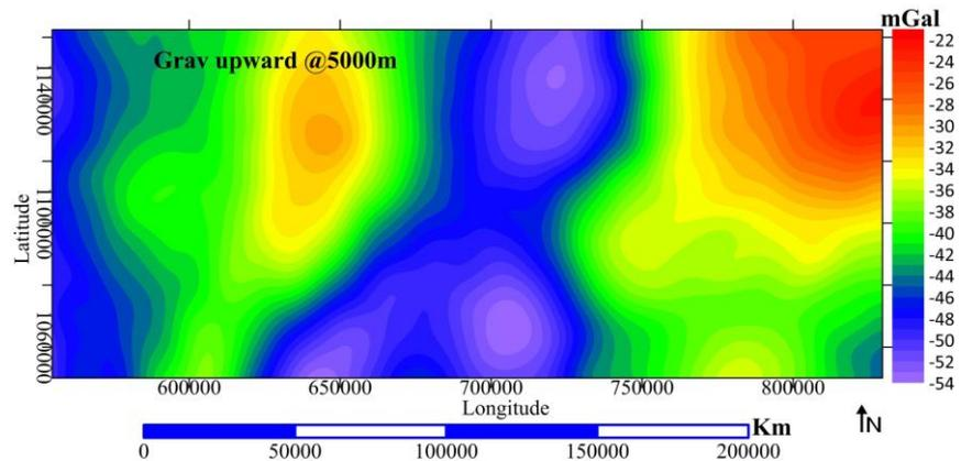
**Figure 8:** Upward Continued Bouguer Gravity Map at 5000m (mgal)
