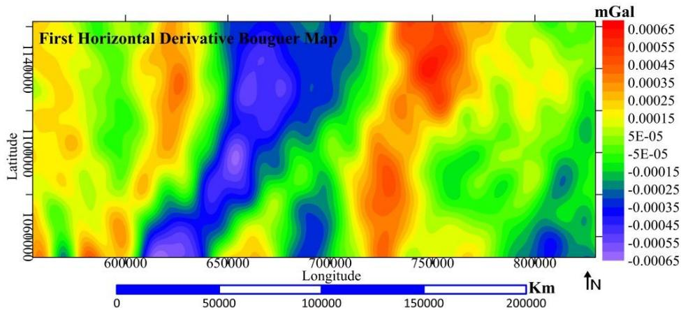
**Figure 6:** First Horizontal bouguer gravity map (mgal)
